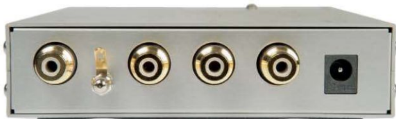
ABOVE: Minimalist back panel filled with high-grade gold-plated phono sockets for signals in/out, the inputs flanking an unnecessarily tiny and fiddly earthing tag; socket at right awaits the forthcoming AC adaptor
